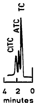
Fig. 1. Separation of TC, ATC and CITC on Perkin-Elmer Sil-X ( 13\ \mu\text{m} ). Column, 5 \times 125\ \text{mm} . Eluent, ( 0.1\ \text{M}\ \text{HClO}_4 + 1.9\ \text{M}\ \text{NaClO}_4 + 0.005\ \text{M} citric acid)-acetonitrile (2:1) (v/v). Eluent velocity, 2.6 mm/sec. Detector, UV photometer, wavelength 280 nm, sensitivity 0.2 absorbance units full scale deflection (a.u.f.s.). Sample about 100 ng of each component.
